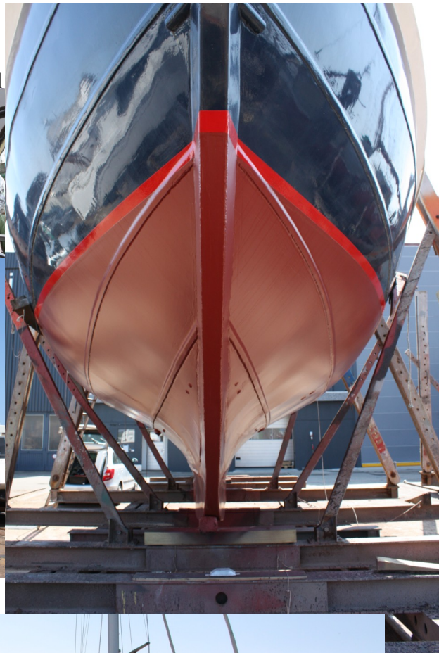
Bottom cleaned to steel and epoxy treated
